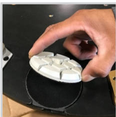
3" Round Resin Tools Mount Fast and Reliably
