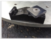
45° Mount for Sharp Cutting Point
