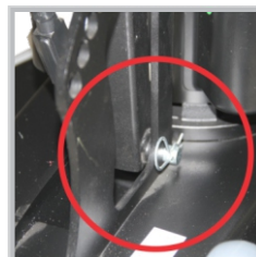
Remove the Handle Mounting Pin w/o Tools
