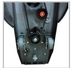
V-Belt Drives Pads at 2000 RPM
