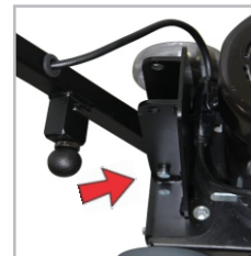
Pull the Pin for Easy Handle Removal
