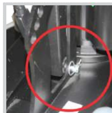
Remove the Handle Mounting Pin w/o Tools
